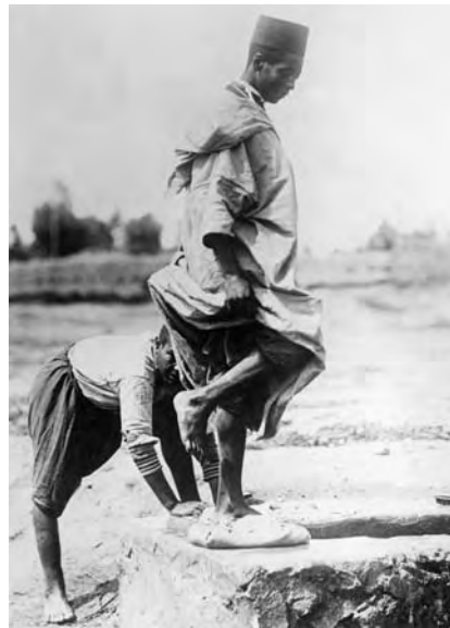
Dyeing the textiles for the traditional cloth of the Moroccans. After the cloth is pulled through the dye, the color is kneaded into the textile using feet. © SVT Bild/Das Fotoarchiv.
