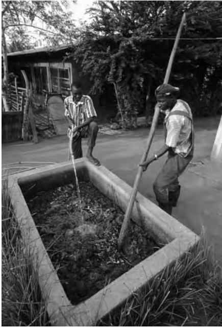
Two students feeding the biogas digester. In the digester, grass, water, and excrement are transformed into biogas and manure. The biogas is stored in tanks and used for cooking and lighting. Benin. © Enrico Bartolucci/Das Fotoarchiv.
