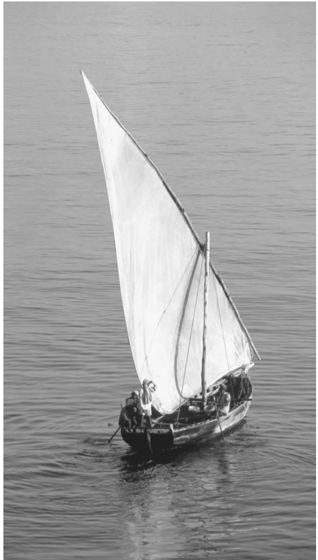
The triangular lateen sail of the dhow, a common sight up and down the Swahili Coast, enabled the ship to steer into the wind. Arab traders used ships of this type to pursue Indian Ocean trade. © David G. Houser/Corbis
