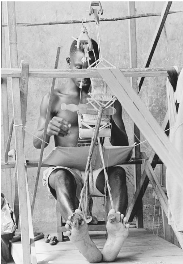
A weaver in the Royal Weavers Village of Bonwire, near Kumasi in modern Ghana, demonstrates how cloth was woven on the traditional heddle loom. The long threads are the warp. © Owen Franken/Corbis
