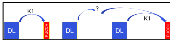
Figure 82. Illustration of the Usage of Non-Numerical K1 for A/N Scheduling
