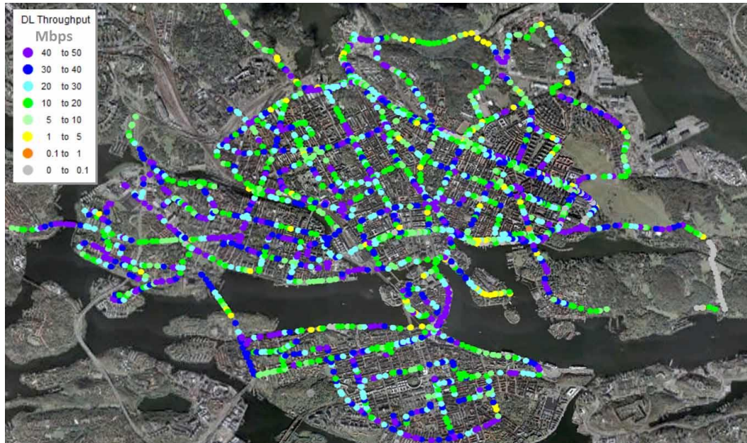
Figure 123: Drive Test of Commercial European LTE Network (10+10 MHz) 289
